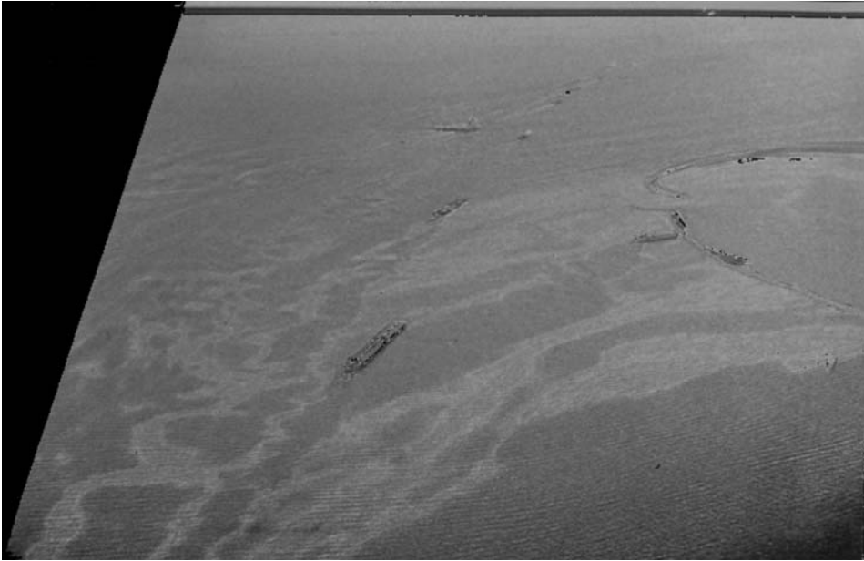
FIGURE 2 A low resolution black-and-white polarimetric image of the oil spill area with the barge located in the lower central portion of the image. The streaming high polarization of the oil distribution is plainly seen in the polarimetric (wideband) image as bright high polarization.
