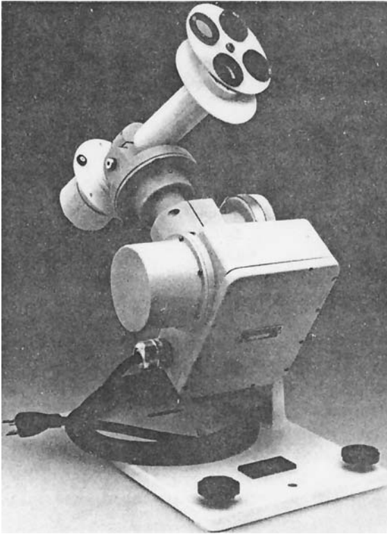
FIGURE 5 Eppley normal incidence photometer.
